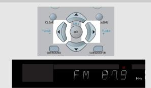
Alternatively, you can press and hold the same button for about one second to activate the automatic search function. In this mode the receiver will automatically tune frequencies until it finds a station.
